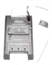
Now you can develop Z-80 based, stand-alone devices such as games, robots, instruments and peripheral controllers, by using your TRS-80 as a development system. The DEVELOP-MATE plugs into the expansion connector of your TRS-80 and adds-PROM PROGRAMMING and INCIRCUIT-EMULATION capabilities to your system (with or without expansion interface).
