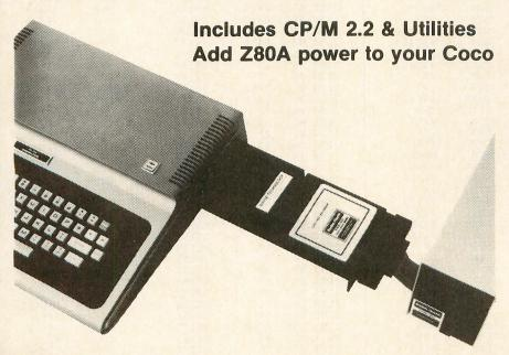
COCO COUPLER 1 is the low cost way to use the world's largest library of personal and professional programs. Simply plug the COCO COUPLER 1 into the expansion port of your TRS-80 Color Computer and plug the disk controller into COCO COUPLER 1 - no modification to your system is needed. COCO COUPLER 1 contains its own 4 Mhz Z80A microprocessor and firmware for efficient execution of CP/M programs. COCO COUPLER 1 supports WORD—PAK 80 x 24 display board from PBJ Inc.
