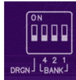
The board includes a 4-position DIP switch that is used to configure which bank of Flash is active at power-up or reset and which addressing scheme is used to communicate with the controller.
