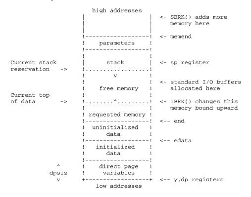
The overall size of this memory area is defined by the "storage size" value stored in the program's module header. This can be overridden to assign the program additional memory if the OS-9 Shell "#" command is used.
